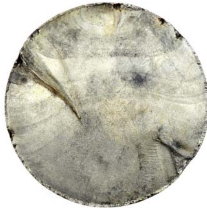
Fracture surface of a shaft that failed due to rotational bending fatigue
