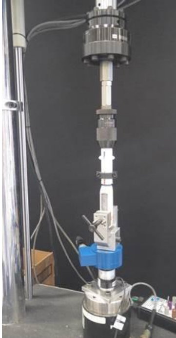
MTS 858 bionix biaxial load frame set up to measure axial and rotational assembly forces
