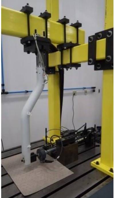
T-slot table configured for testing a medical equipment ceiling suspension system
