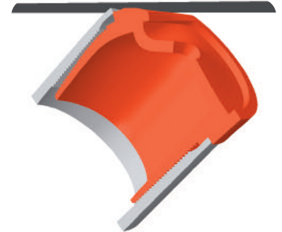
A computer simulation of an angular impact test. The box thread protector and coupling box are shown in cross-section at the end of the impact.
