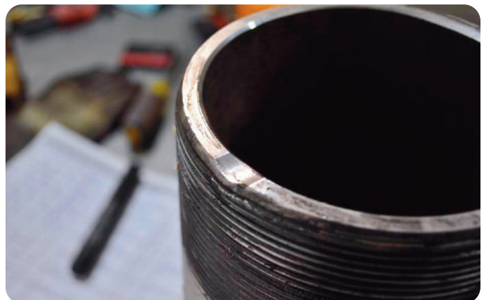
Damaged pin from axial impact test.
