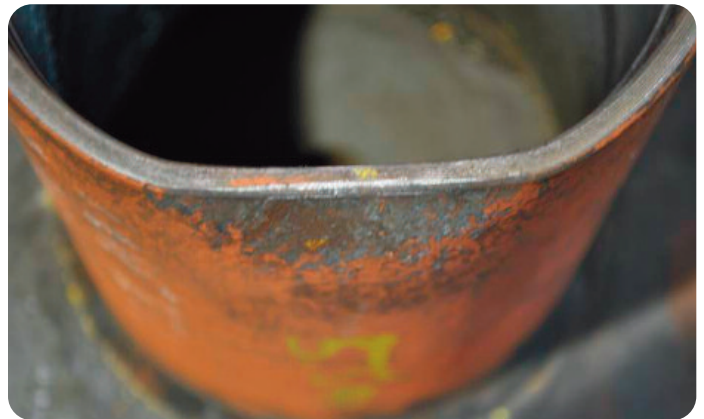
Damage coupling from angular impact test.
