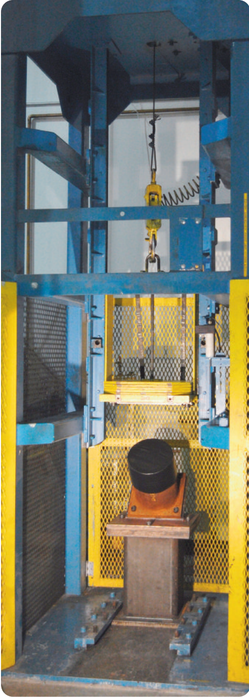
SES Thread Protector Impact Load Frame with 45 degree angle drop fixture installed.
