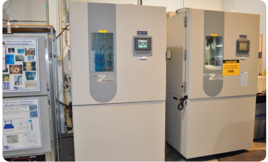
Environmental conditioning chambers with -50°F to 375°F thermal range.
