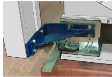
*A digital twin of the retort system was used to identify the actual load path through the pedestals into the foundation. Once designed, each pedestal was calibrated in a load frame in our laboratory. The completed sensors were installed on the retort system to collect data in real-time.*
