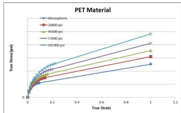
Figure 4: PET material stress-strain curves as a function of HPP hydrostatic pressure
