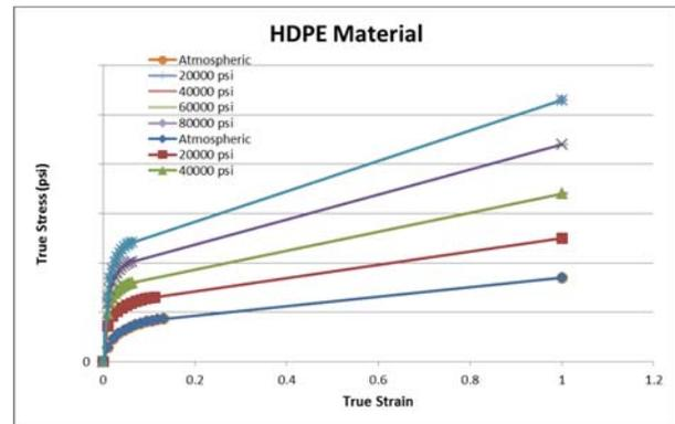
Figure 3: HDPE material stress-strain curve as a function of HPP hydrostatic pressure
