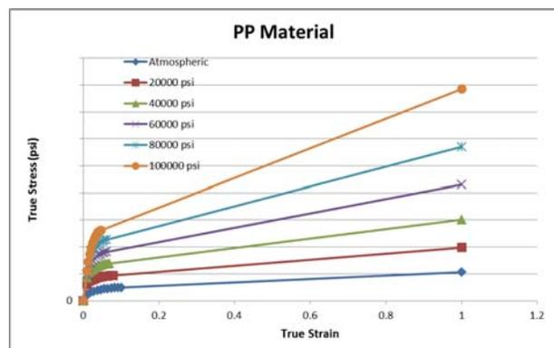
Figure 5: PP material stress-strain curves as a function of HPP hydrostatic pressure
