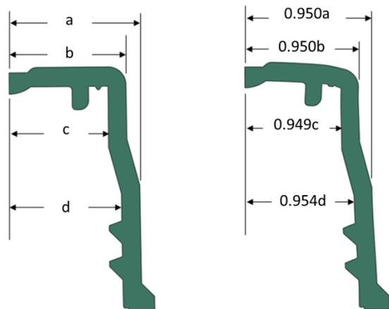
**Figure 8: Predicted change in closure dimensions as a result of HPP processing (left – original, right – change)**
