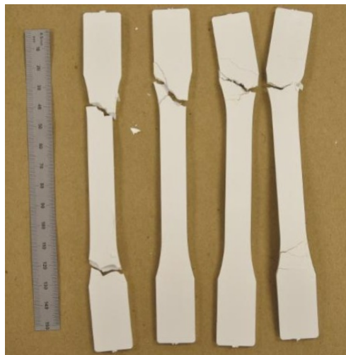
ABS test specimens cracked by exposure to a quaternary disinfectant
