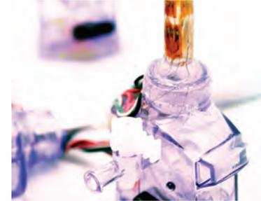
This trocar has been instrumented with strain gauges to determine the loads it experiences during a simulated surgery. Once determined, this data becomes a driver for the design requirements of future devices.
