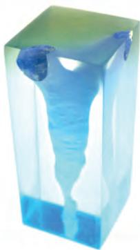
This model, created from a CT scan, was used to guide sizing calculations for a device designed to operate on the vocal folds of pediatric patients.
