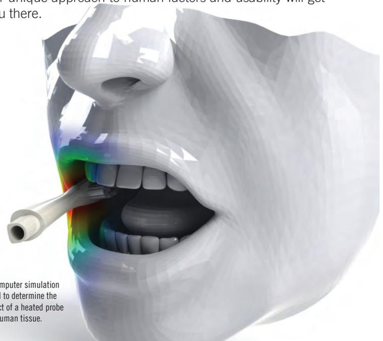
A computer simulation used to determine the effect of a heated probe on human tissue.
